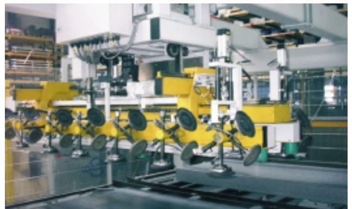
automatic width and length adjustment of suction crossbeam
