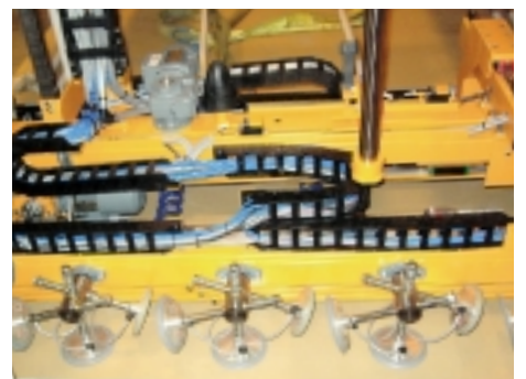
fully automatic length adjustment of suction traverse
