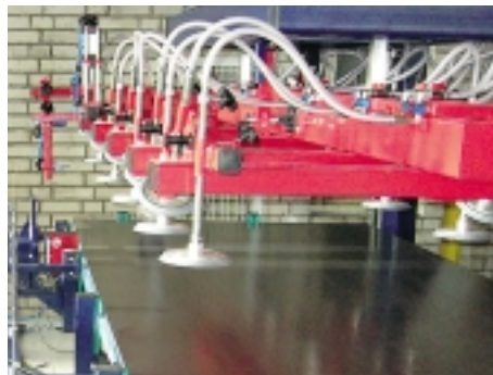
with fanning magnet for steel sheets
