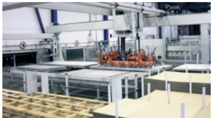
fully automatic 3-axle-portal
