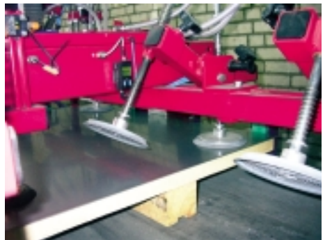
manual change of cups with compensator
