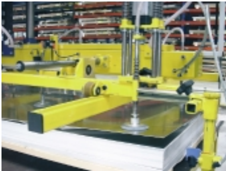
automatic sheet separation
