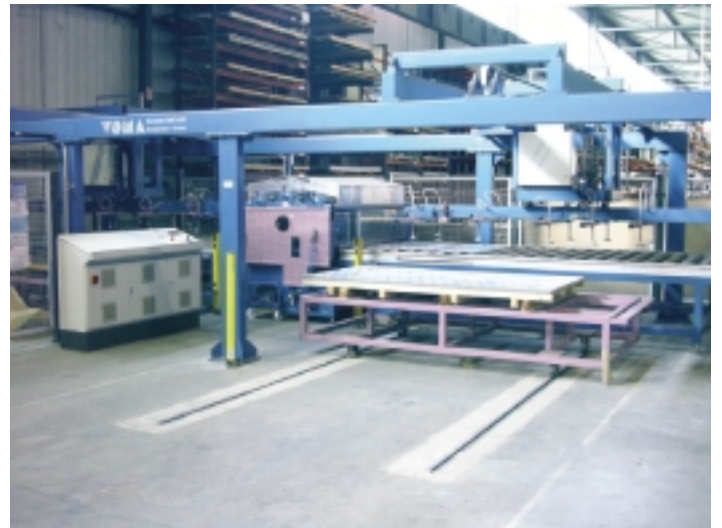
fully automatic laminating line one-man control
