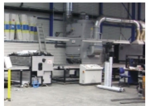
combined grinding- / brushing line
